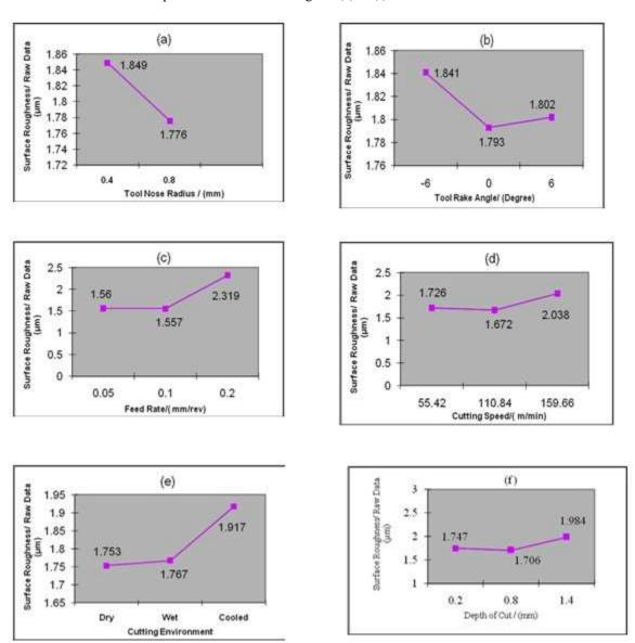
Fig 4.1: Response graph of surface roughness (a) effect of tool nose radius (b) effect of tool rake angle (c) effect of feed rate (d) effect of cutting speed (e) effect of cutting environment (dry, wet, cooled) (f) effect of depth of cut.
